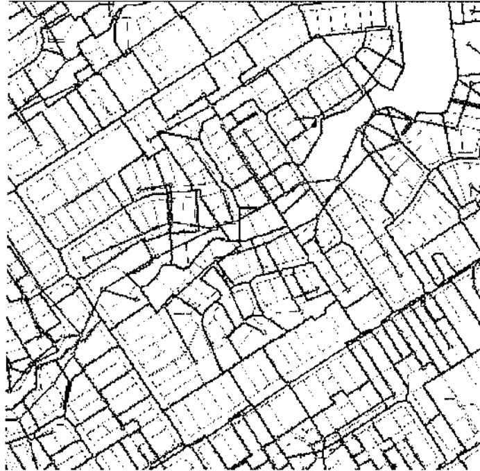
Figure 5-3 Example of detailed catchment delineation using the double sweep Thiessen Polygon Method
