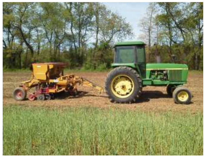
This no-till drill, is available for farmers to borrow from the Conservation District in order to implement this best management practice (BMP), which reduces erosion and nutrient pollution to local waterways, without having to purchase their own equipment to try the BMP. The drill was purchased through the County’s National Fish and Wildlife Foundation Grant, administered by the Planning Department.
