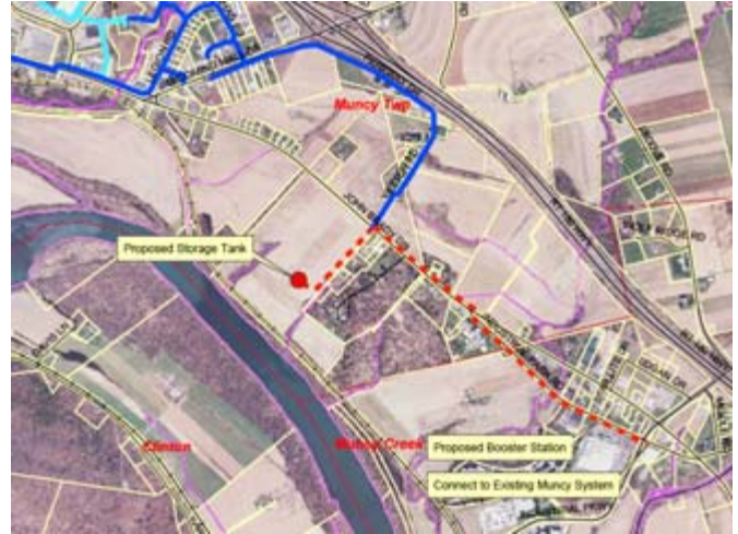
Phase II of the Halls Station water system includes the Muncy Interconnector (shown in red)
