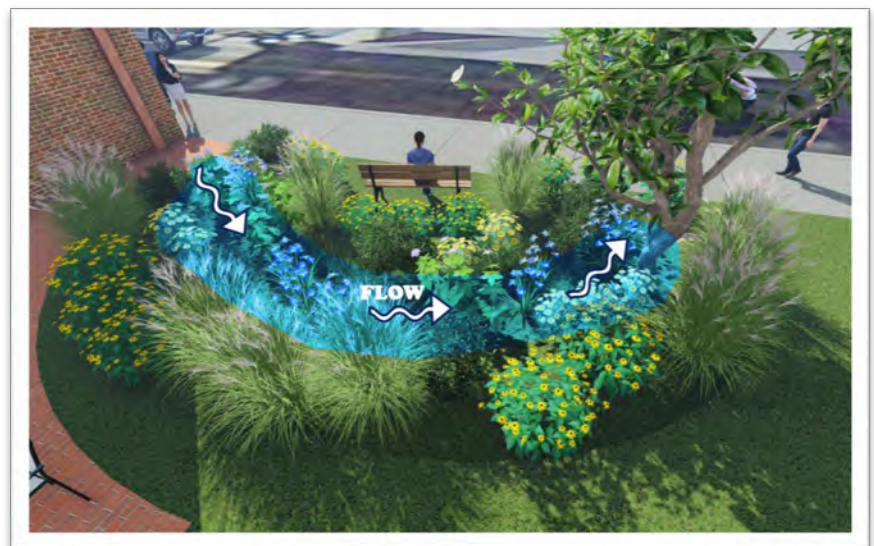
Stormwater flow into rain garden Source: Larson Design Group
